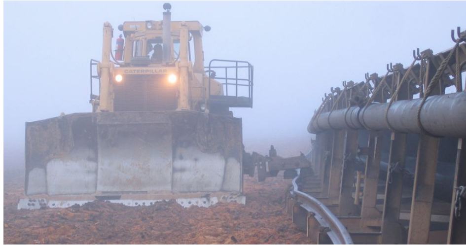
■ Figure 4-2 – Conveyor track shifting bulldozer in operation.
