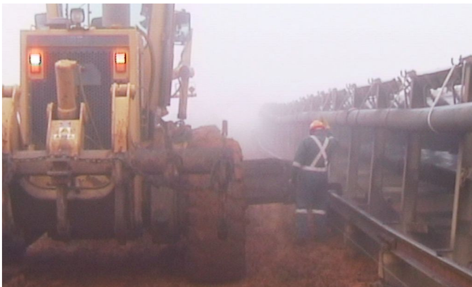
■ Figure 4-3 – Final conveyor alignment after track shifting would be achieved using a grader.
